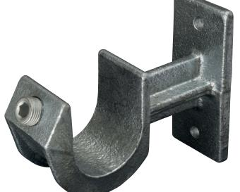
A wall mounting handrail bracket, the tube simply drops into this hook fitting and is secured with the grub screw.
