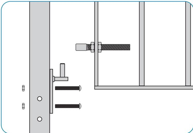
Fit one of the bolt on hinge pins to the lower section of the hinge post and fit to gate eye.
