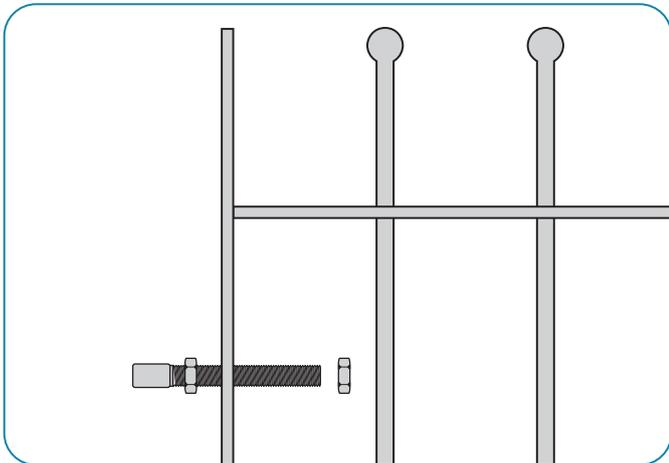
Fit one of the adjustable gate eyes to the top corner on the hinge side of the gate.
