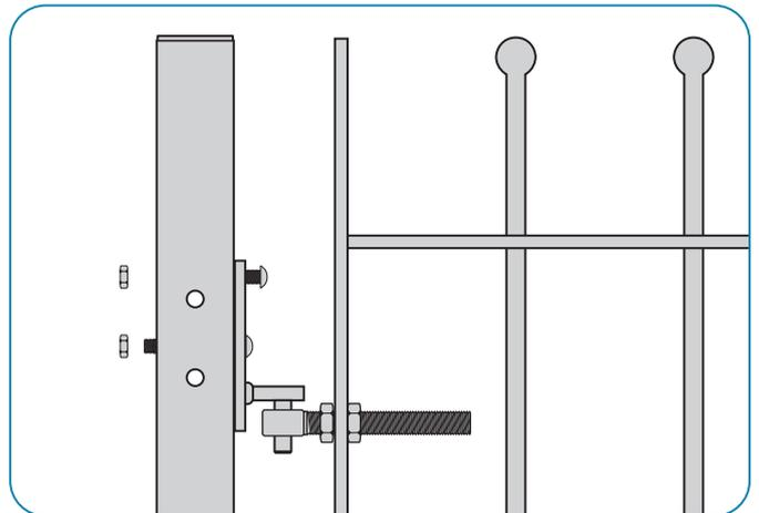
Fit the other gate pin through the upper gate eye and secure to the post.
