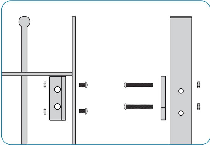
Bolt the latch keep to the post and the latch holder to the gate.
