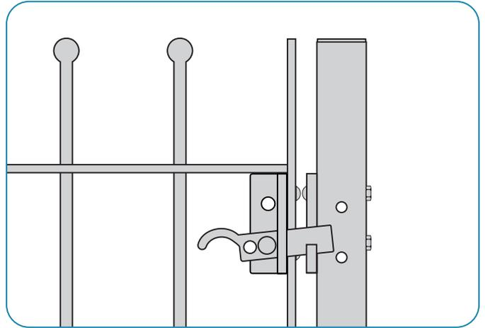
Bolt the latch to the latch holder, don't over tighten so that the latch can move easily.
