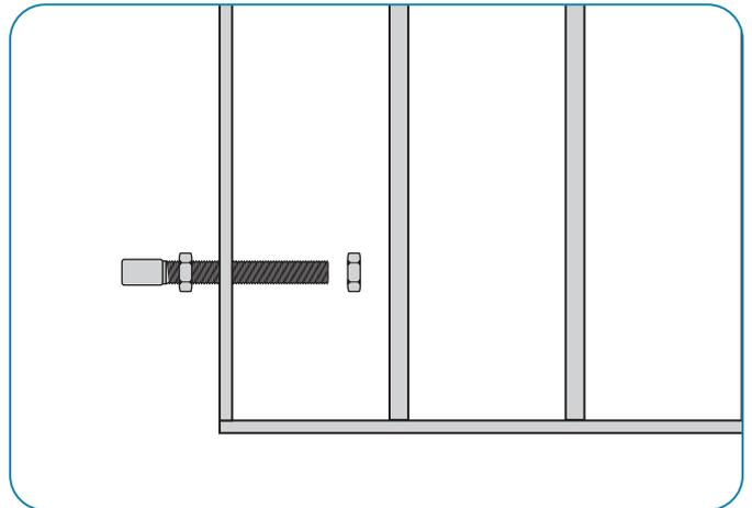
Fit the other adjustable gate eye to the bottom corner of the gate.
