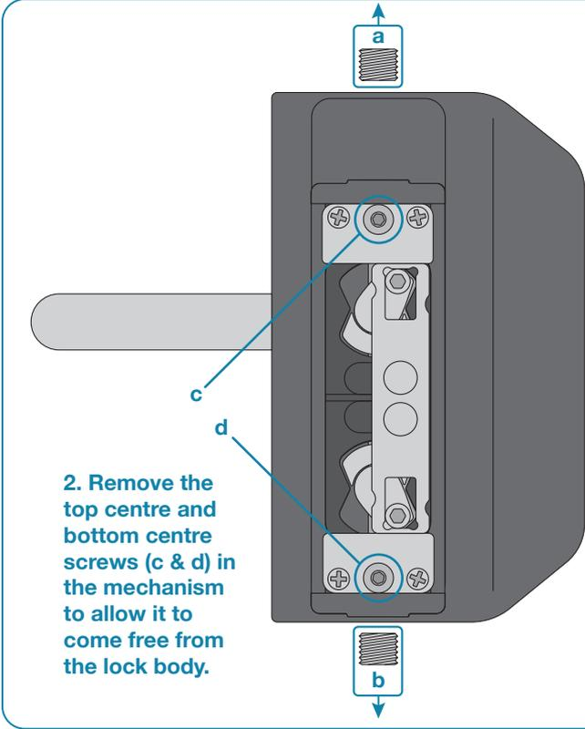
1. Remove the two grub screws (a & b) on the top and bottom of the paddle hinge. This will allow the hinge pin to come free and the paddle to be removed exposing the mechanism.
