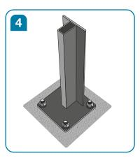
Tighten the fixing bolts down with a hex spanner, making sure that the post base is level as you do this.
