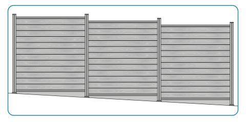
On slopping sites we recommend the use of a gravel board under the base rail.
