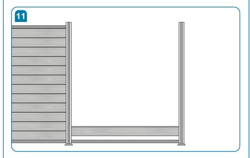
Slide the first fence board into the top of both posts and lower down onto the tongue of the lower rail, check this is still level.
