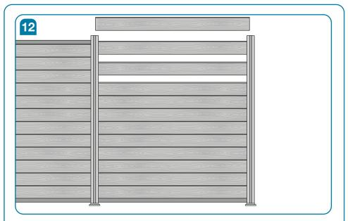
You can now fit the rest of the fence boards into place using the tongues and groves on each board.
