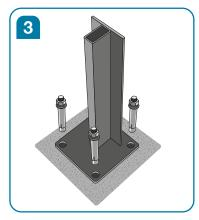
Set the post base over the holes and insert the fixing anchor bolts. The post base is a T section, make sure the top bar of the T is running in the same direction as your fence line.
