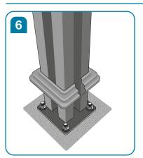
Fit the protective weather shield over the post base to keep the elements at bay and protect the fixing bolts, making sure to remove the push out section that accommodates the bottom rail.
