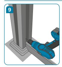
Drill 6mm pilot holes through the holes in the L bracket into the post. Secure it to the post with the screws provided.
