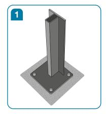
Once your foundation pads are dry, position your post base in the centre of the pad and mark out the fixing hole positions. If you are concreting in your posts skip to stage 6.
