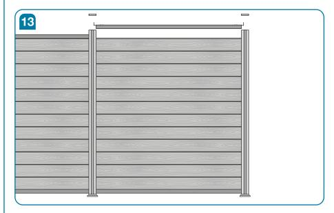
Now fit the top rail into place and secure with the L brackets and screws provided, the post caps can now be fitted.
