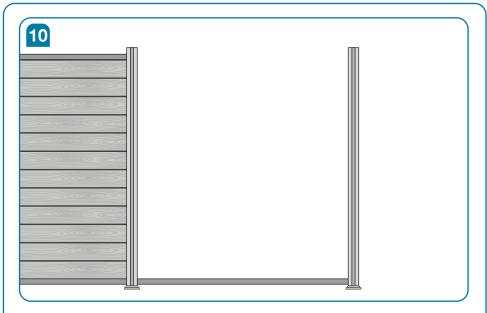
Once the base rail is fitted securely between two posts you are ready to start fitting the fence boards which should be cut to 1750mm wide.
