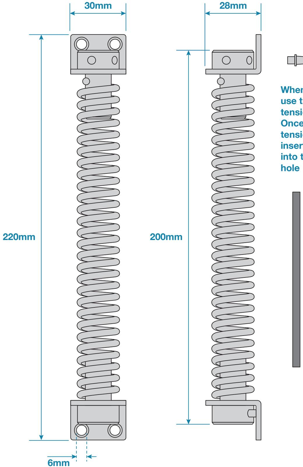
**When fitted to gate use the bar to tension the spring. Once the required tension is found insert the locking pin into the appropriate hole**
