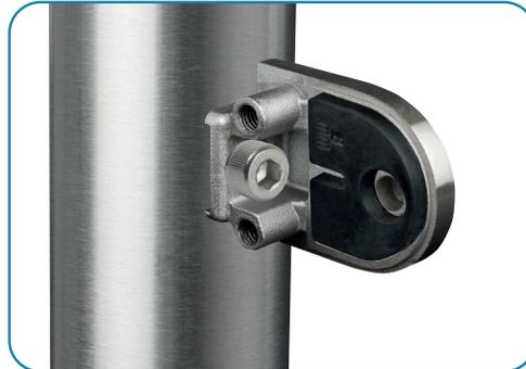
With your glass temporarily supported in the desired position fit the second rubber gasket and the other half of the glass clamp (if using the glass support pin your glass will need to be drilled prior to this). Fix with the two supplied hex head countersunk screws.
