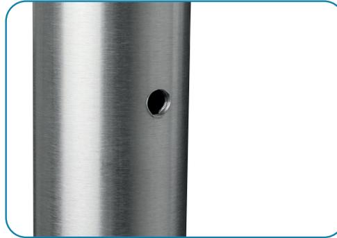
Fix half of the glass clamp to the post with an M8 hex head fixing screw. (available separately code: SSA11820). Tighten with a hex head bit or allen key.
