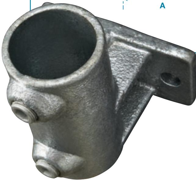
A non structural offset side palm base fitting for fixing level or sloping guardrail to walls, steps ramps etc. The tube is unable to pass through this fitting as supplied, should this be required then the base must be reamed out.
