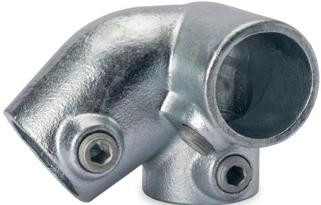
A top sloping left hand elbow fitting designed for top rail on slopes & staircases between 30° & 45° at the junction where the handrail changes from level to sloping down.
