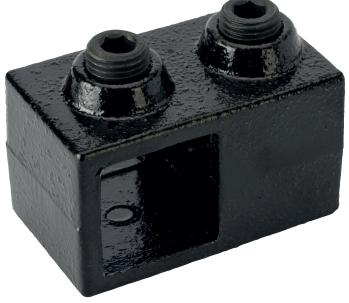
A 90° short tee connection between 2 tubes, typical use is on straight and level guardrail to connect the vertical post to the top rail or end/mid rail. It cannot be used to join tubes in the top of the short tee, to join tubes use the 104 long tee.
