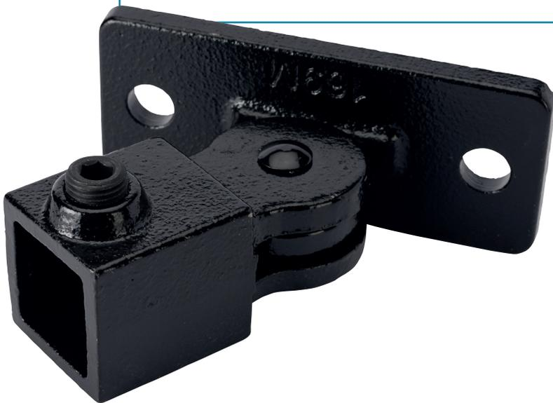
A swivel fitting, ideal for fitting angled tubes to walls, the swivel has a travel of approximately 85° from the vertical in each direction, it should never be used as base fitting for guardrail systems.
