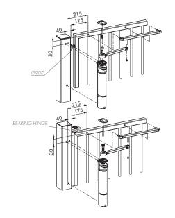
Order code • VERTICLOSE-RAIL • With arm and rail for 90° hinge situations
