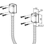
This Stainless steel cable guide is the best way to get power into a swing gate and to protect your electrical wires in an outside environment.
