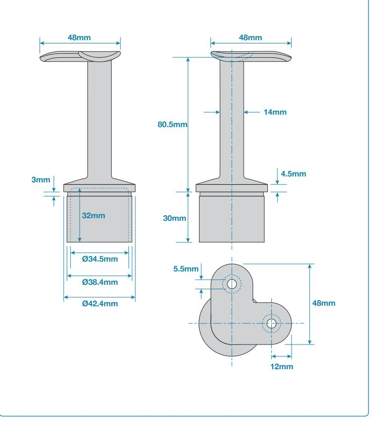
**Stainless Steel 304 Tube To Tube** 90° Handrail Support To Suit 42.4 x 2mm Tube & 42.4mm Handrail code: S4HS922
