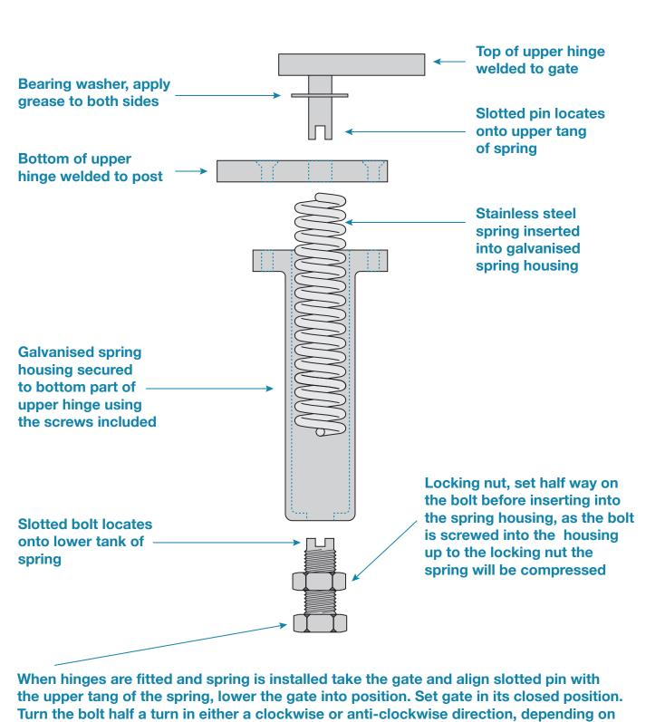
the desired direction of swing. Over tension will damage the spring.
