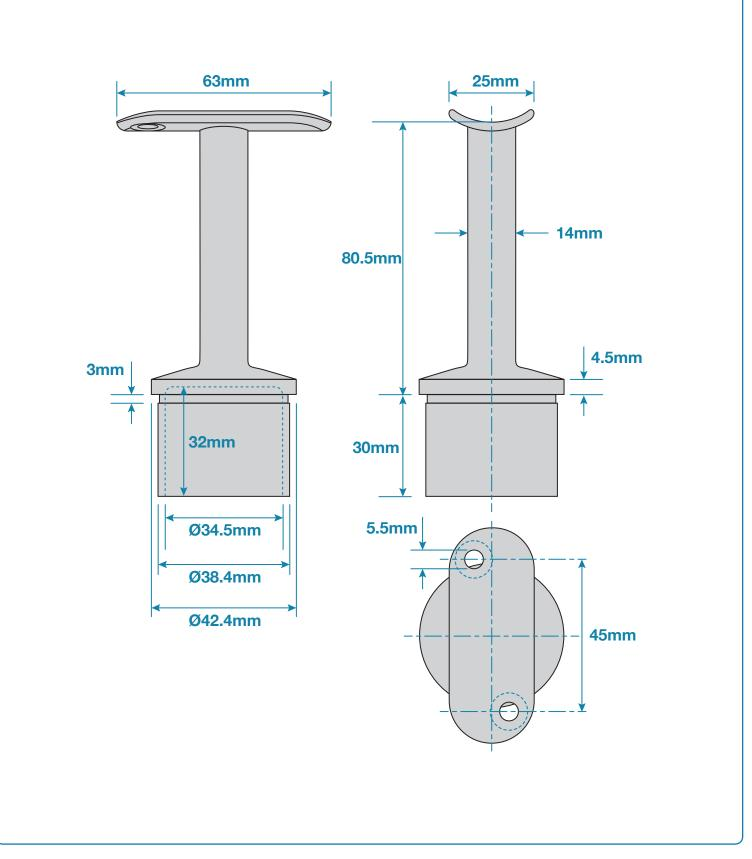
Stainless Steel 316 Tube To Tube Handrail Support To Suit 42.4 x 2mm Tube & 42.4mm Handrail
