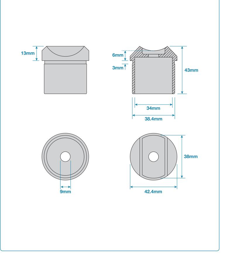
**DC** Iron **Stainless Steel 316 Tube Saddle** for 42.4 x 2mm Tube code: SSHS30242
