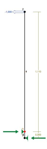
Determination of the forces acting on the insert, which transfer the load on profile walls (characteristic loads):
