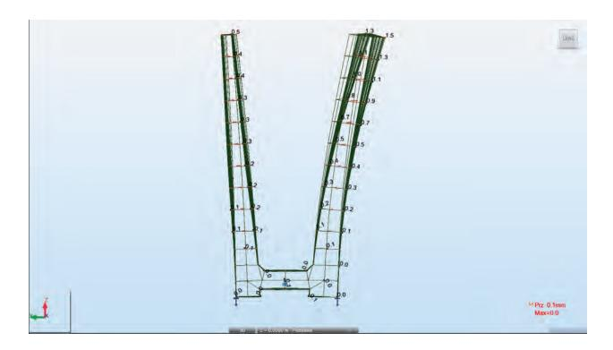
The maximum deflection of the vertical wall profile is 1,5mm.
