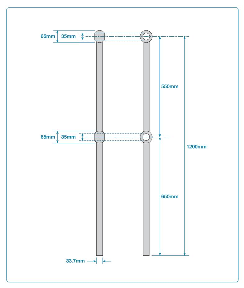
Mild Steel Tubular Handrail Standards To Suit 33.7mm Rail
