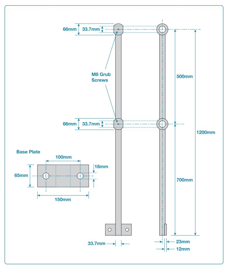
Galvanised Handrail Standard With Side Palm To Suit Tube 33.7mm
