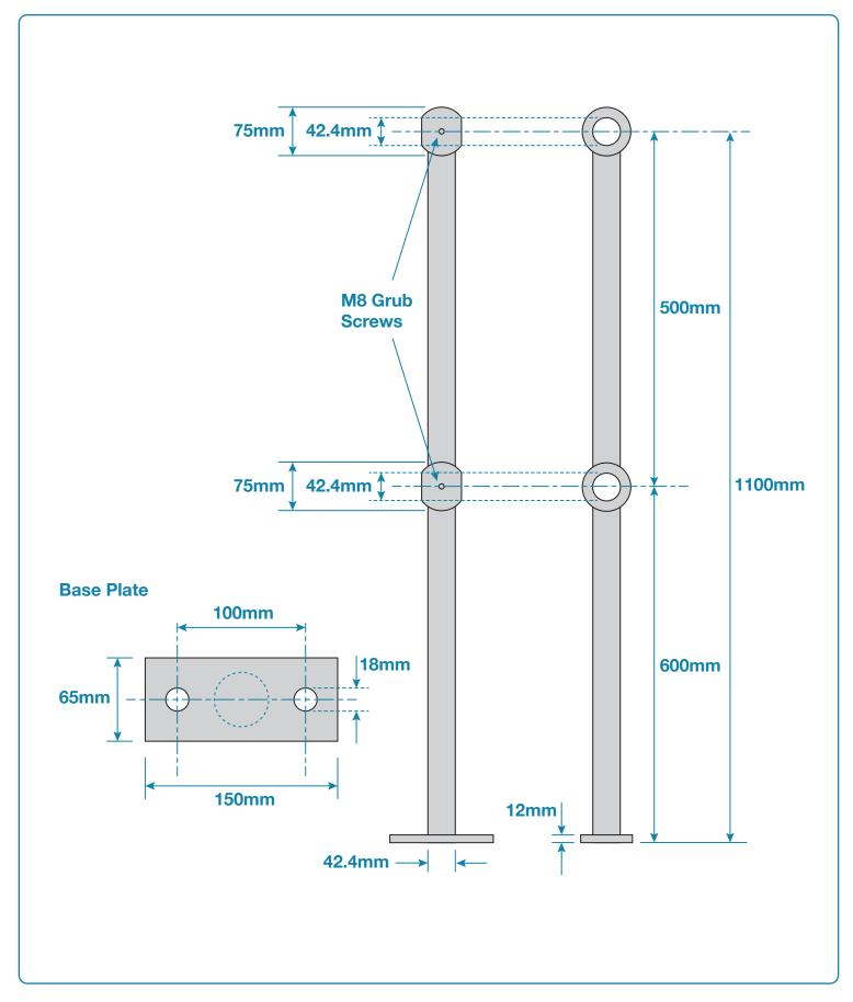
Galvanised Handrail Standard With Flat Base To Suit Tube 42.4mm
