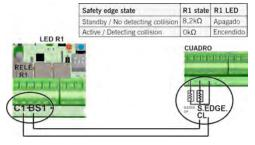
The equipment can be connected to the control panel with input for safety edge 8k2 or directly into a safety input normally closed contact as if it were a photocell or stop signal.
