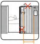
In installation likely to have communication cuts between the transmitter and the receiver, the antenna must stand vertically from the hole in the gland.
