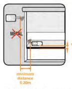
Do not place metal surfaces between transmitter and receiver.
